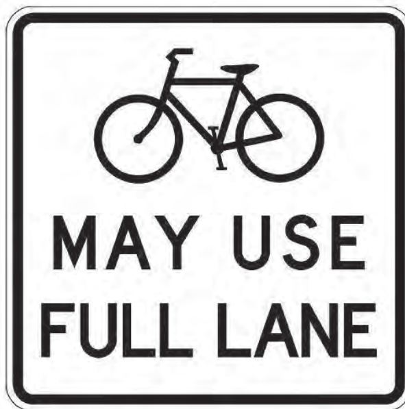
"Bikes May Use Full Lane" (R4-11) sign from the Manual on Uniform Traffic Control Devices (MUTCD)
